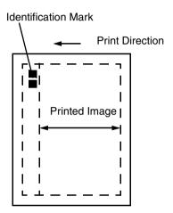
The printable area is reduced by 3 mm on the left side and the 1.5-mmwide identification mark is printed in the top corner of the page at a distance of 1.5 mm to the left of the image.
